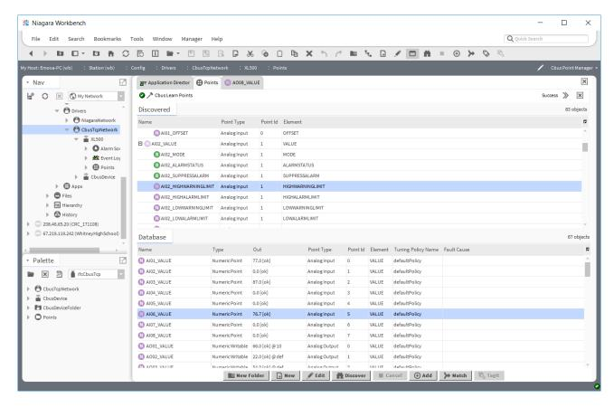
Single or multiple points can be added as control points with CbusProxyExt extensions by selecting the discovered row(s) in the top pane, and clicking add. Doing so will cause the "Add" dialog box to appear: Once the point(s) are satisfactorily edited, click "OK" to create the proxy points corresponding to the point property.
