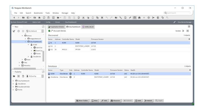
Single or multiple Cbus devices can be added as device by selecting the discovered row(s) in the top pane, and clicking add. Doing so will cause the "Add" dialog box to appear: Once the device(s) are satisfactorily edited, click "OK" to create the device corresponding to the device property.
