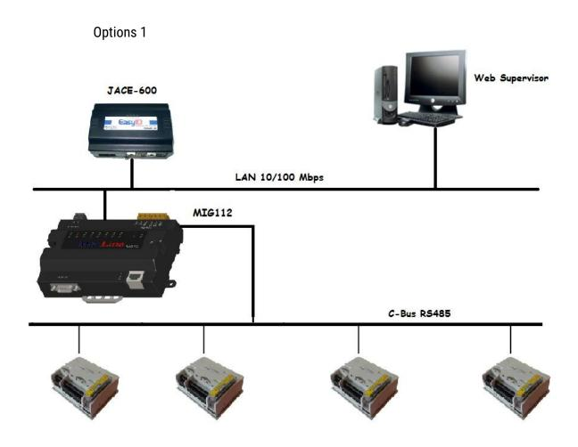
Note: Make sure the Cbus RS485 connection is connected at the terminal D2+/D2-:-
