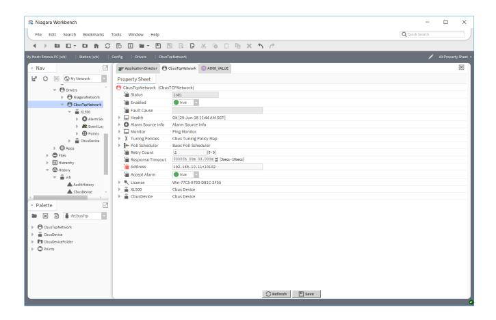
The alarm point can define at the Cbus Proxy Extension, simply select the "Alarm Class" property and select from the existing alarm class list and the alarm will automatically route to the selected alarm class.
